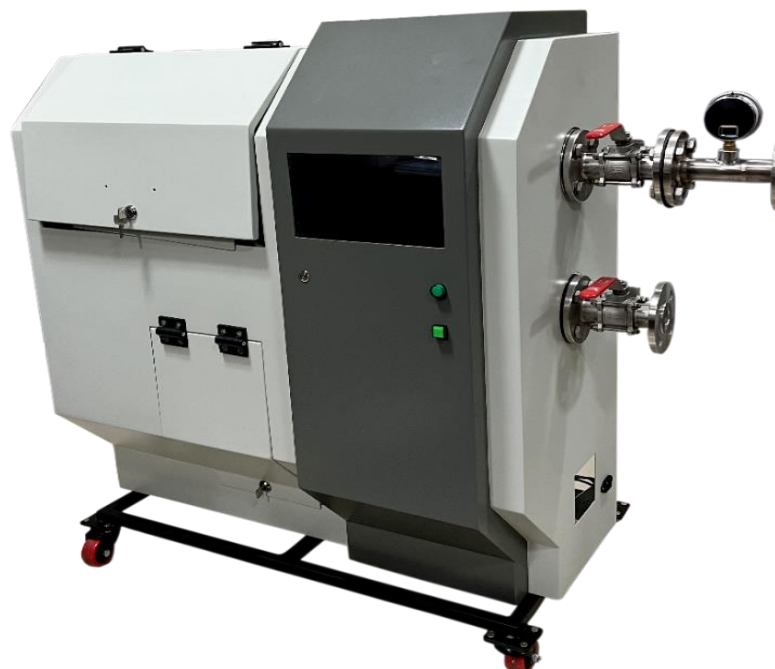
Fig. 1. OSIS- Online sucro crystal imaging system
